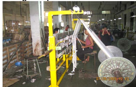
(2) Drawing the warp beam ready for weaving
