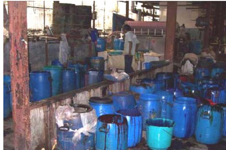
Chemicals without any covering
